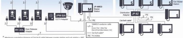
\* Maximum cumulative distance of Cat-5e/6 cable between master station and sub station = 980'
