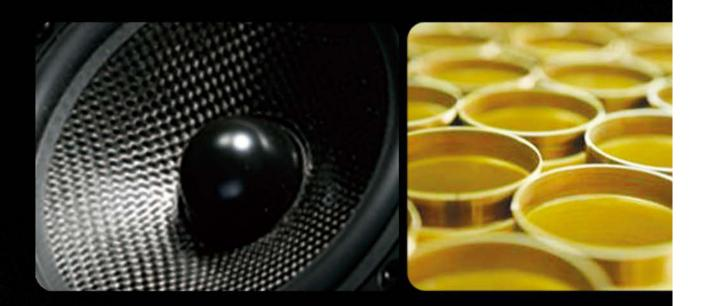
Castle's famous carbon fibre woven cone is retained as it offers exceptional strength to mass ratio, operating as a pure piston over its pass band. The motor system utilizes a Kapton former with a copper clad aluminium voice coil to achieve a wide bandwidth into the treble region. Built onto a Castle classic cast alloy chassis, this 110mm unit offers a remarkable bandwidth and superb dynamic performance.
